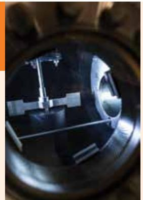
Close-up view of the high-speed propeller inside the injector.
