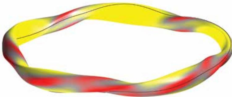
*Magnetic field strength in a turbulence-optimized stellarator design. Regions with the highest strength are shown in yellow.*
